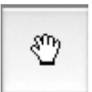
This tool, also known as the grabber, is used to drag the plan view to focus on another part of the plan. A shortcut to this tool is to hold down the option key on Macintosh, or the right Alt key on Windows. This shortcut is available at any time, such as when you have another tool active.
