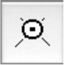
New IP (Intersection Point) is added where you click with this tool. The new IP will be added to the end of the active control line. Before choosing this tool, be sure to make active the control line to which you want to add an IP. Use this tool in conjunction with road control lines
