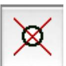
This dodgy looking tool is used to delete an IP of the active control line. Place the cursor over the IP you wish to delete and click.
